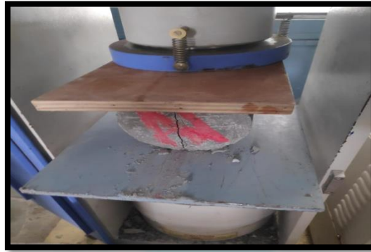
Figure 6: Split Tensile Strength Test Setup.
