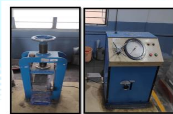
Figure 7: Flexural Strength Test Setup.
